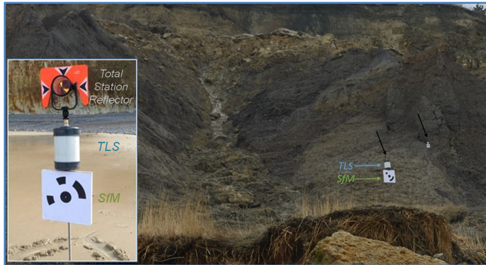
Fig. 5 Setup of the used Ground control point to georeference both the SfM and TLS models
