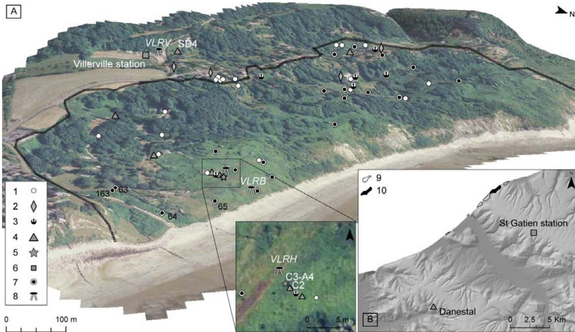
Figure 2. Monitoring network for the Cirque des Graves landslide. A: Cirque des Graves landslide. B: Pays d'Auge Plateau. 1: Piezometer; 2: wells; 3: Inclinometer; 4: Piezometer with permanent sensor; 5: Geobead probe; 6: Meteorological station; 7: Topographic benchmark, 8: Permanent GNSS receivers; 9: Active landslide; 10: Cirque des Graves landslide.
