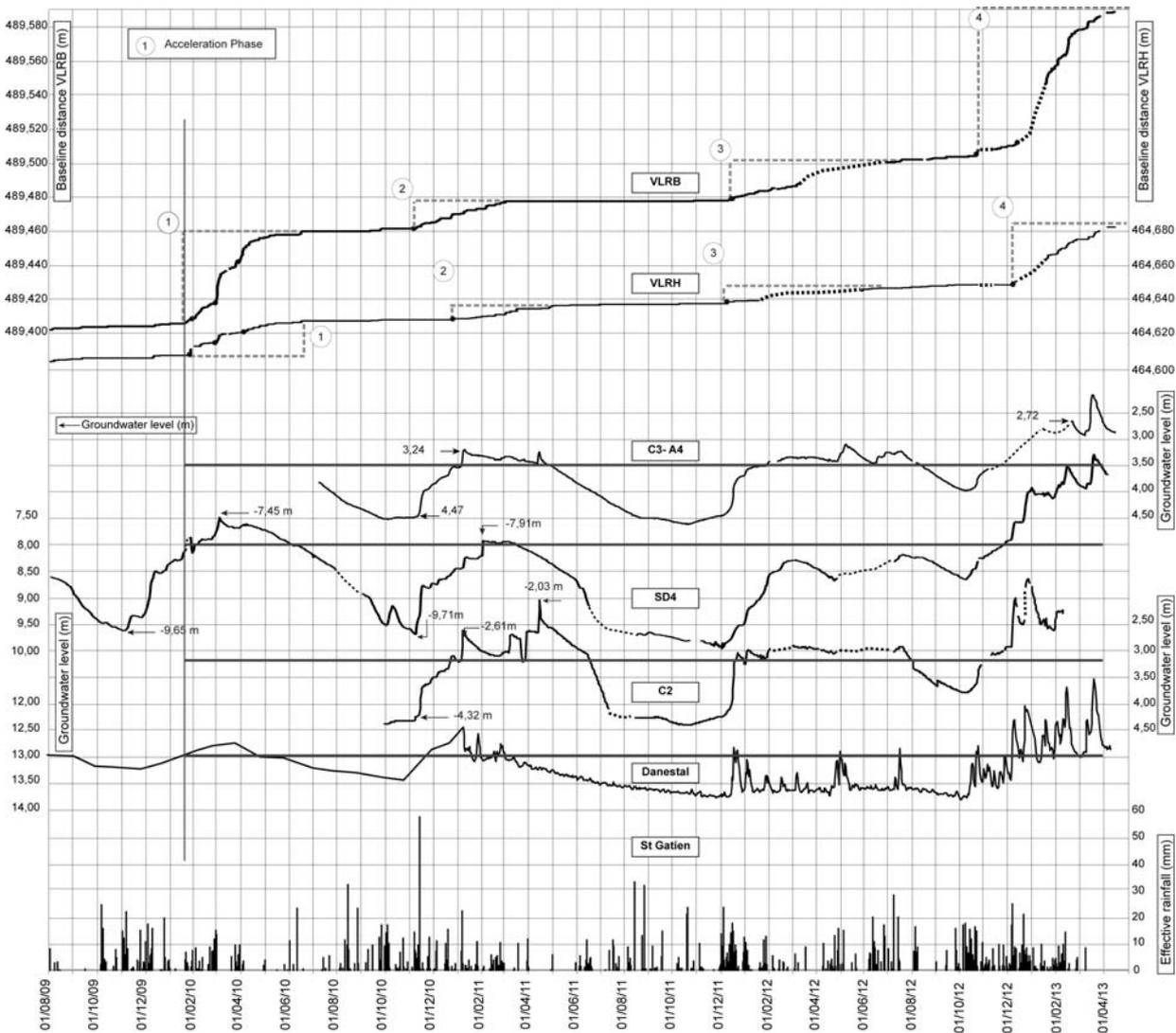
Figure 4. Relations between the displacements (GNSS VLRH and VLRB), piezometric levels (SD4 and C2), pore pressure (A4) recorded at Cirque Graves and daily rainfall of St Gaten station
