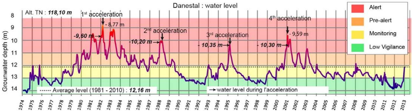
Figure 3. Groundwater level at Danestal since 1974 and critical water level for warning system
