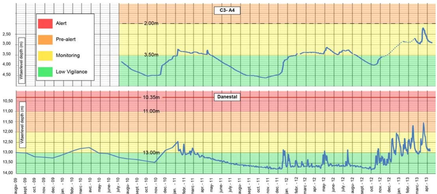
Figure 5. Groundwater levels at Danestal since august 2009 and A4 since august 2010 and critical water level for warning system
