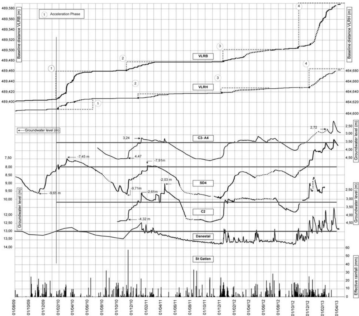
Figure 4. Relations between the displacements (GNSS VLRH and VLRB), piezometric levels (SD4 and C2), pore pressure (A4) recorded at Cirque Graves and daily rainfall of St Gation station
