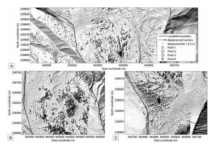
Figure 10. Displacement field for the 20<sup>th</sup> May 2008 in the local coordinate system in the upper part (A), in the middle part (B) and in the lower part (C) of the mudslide. The trajectories of the points 1, 2, 3 and 4 are also shown. Their cumulated displacements are presented in Figure 8.
