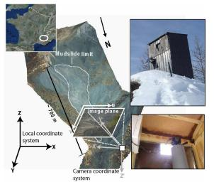
Figure 1.View of the Super-Sauze mudslide, the camera monitoring system and the different coordinates system involved in the georeferencing procedure.
