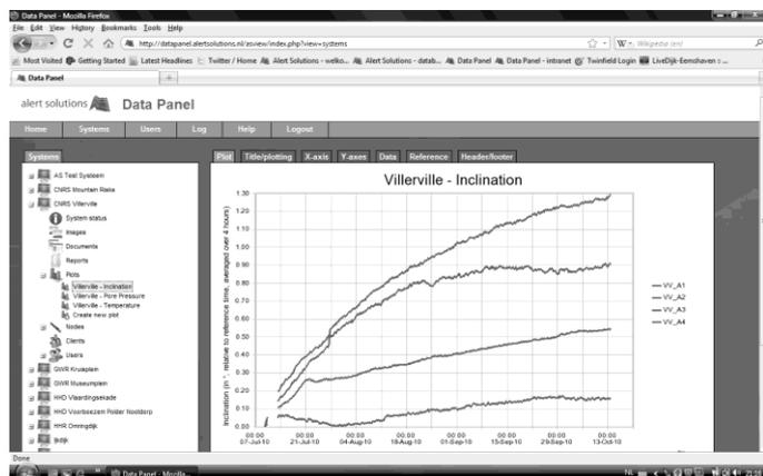
Figure 2. A web application gives worldwide instant access to measurement data and analysis results from all monitored sites.
