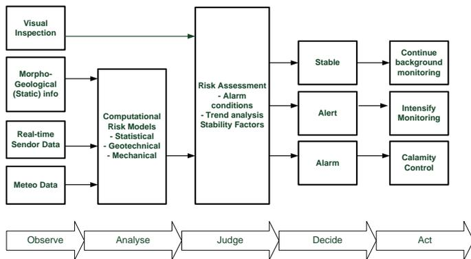
Figure 4. Flow diagram depicting elements of an early warning system applying real-time monitoring in order to continuously update stability calculations and assessment of alarm threshold conditions.
