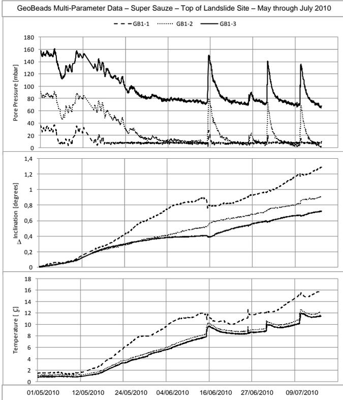
Figure 3. GeoBeads multi-parameter measurements from the installation at the top of the Super-Sauze mudslide over the period May to July 2010. From top to bottom graph, 1) pore water pressure [mbar], 2) delta inclination [degrees], and 3) temperature [°C]. Sharp pore water pressure peaks (top graph) coincide with observable inclination trend changes and temperature increases in the lower layers.
