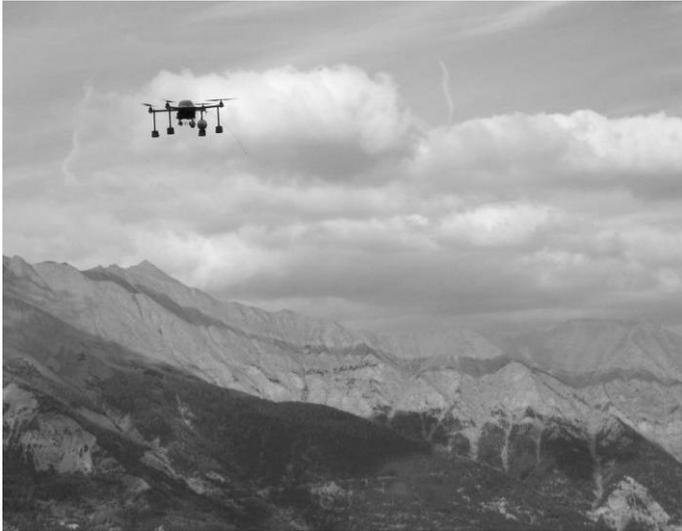
Figure 1. Quad-rotor for remote controlled picture surveys.
