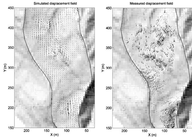
Major cumulated displacements are directly correlated with areas where the thickness of the layer C1 is important (Figure 8) (middle part and lower part).
