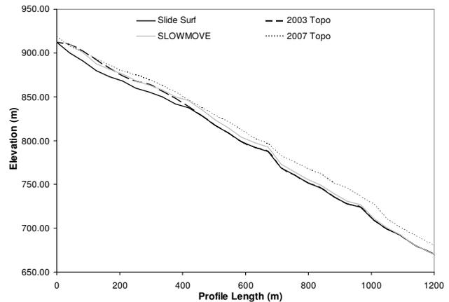
Figure 6. Results of topographic reconstruction after 1000 days. The SLOWMOVE acronym represents the implemented numerical model
