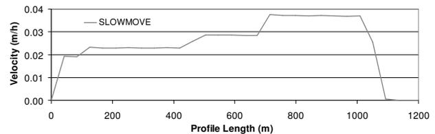
Table 4. Results of a simulation of a cross section of the Valoria landslide (1000 days).
