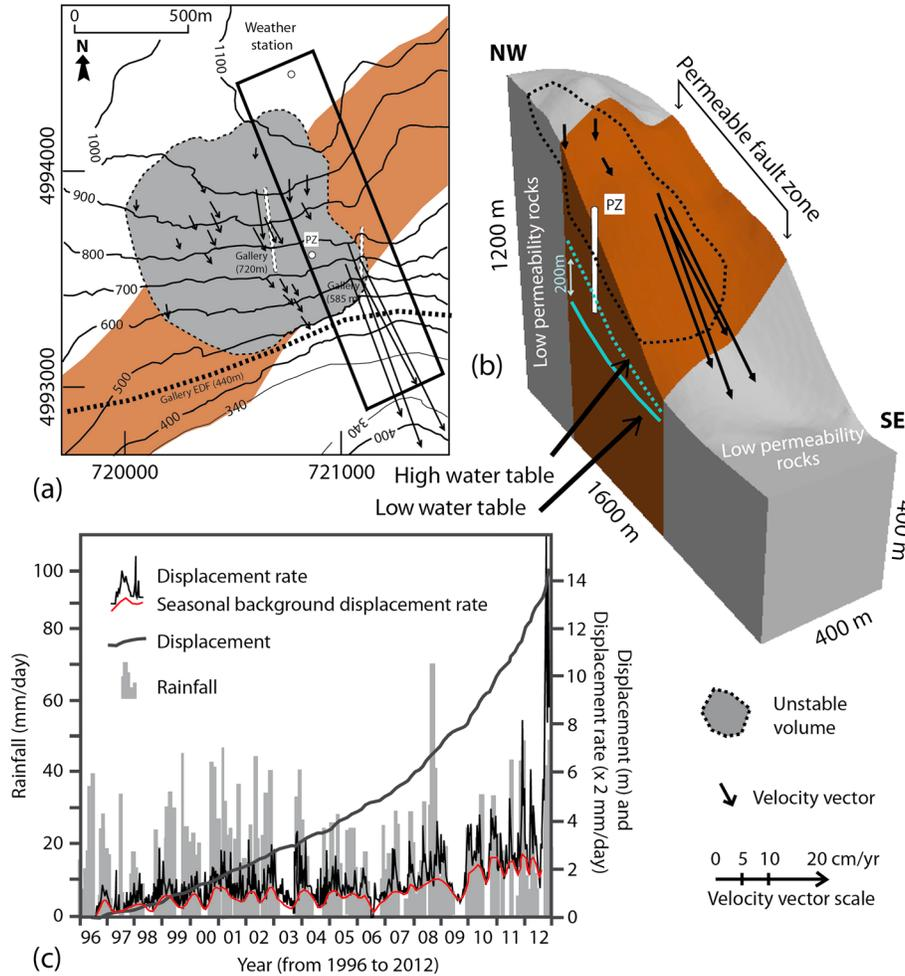
**Figure 1.** (a) Simplified geological map showing the location of the Séchilienne landslide and the displacement vectors. The black solid rectangle on the map illustrates the location of the (b) three-dimensional view of the high-motion zone and the position of water table (PZ is the piezometer). (c) Pluriannual variations of landslide motions compared to effective rainfall events. (Detrended seasonal variations were obtained from *Vallet et al.* [2013]).
