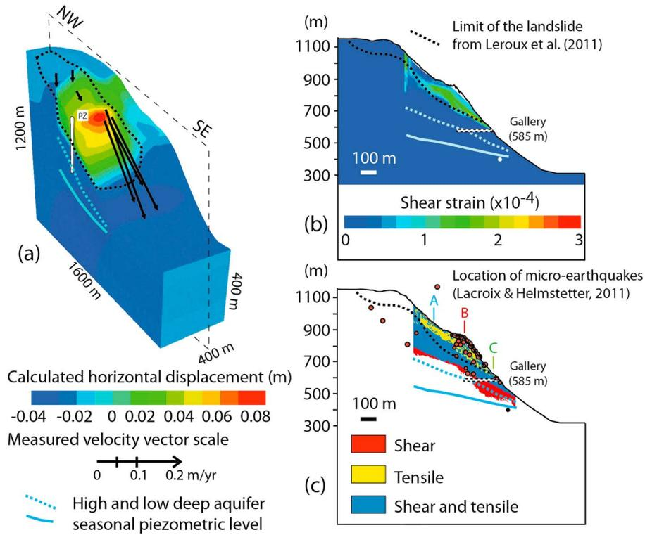
**Figure 2.** Comparison of model results to geodetic, geophysical imaging, and microseismic data. Three-dimensional views of (a) horizontal displacements, (b) shear strain, and (c) plastic rupture plotted on the NW-SE cross section in Figure 2a (indexes A, B, and C indicate the location of measured vertical profiles presented in Figure 3).
