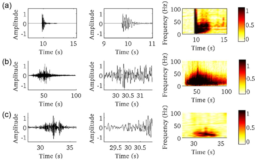
**Figure 2.** (Left) Seismic events recorded by sensor 1 of station THE, (middle) zoom over a 2-s window at the beginning of the signal, and (right) corresponding time–frequency diagram. All amplitudes have been normalized to the peak values. From top to bottom: (a) a shot, (b) a rockfall that occurred on 28 October 2008, (c) a local microearthquake that occurred on 29 October 2008. The color version of this figure is available only in the electronic edition.
