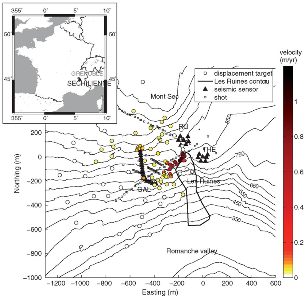
**Figure 1.** Map of the Séchilienne rockslide. Filled circles show the position and velocity of displacement targets. Open squares show the location of shots realized for tomographic purpose. Seismometers are shown as black triangles. The color version of this figure is available only in the electronic edition.
