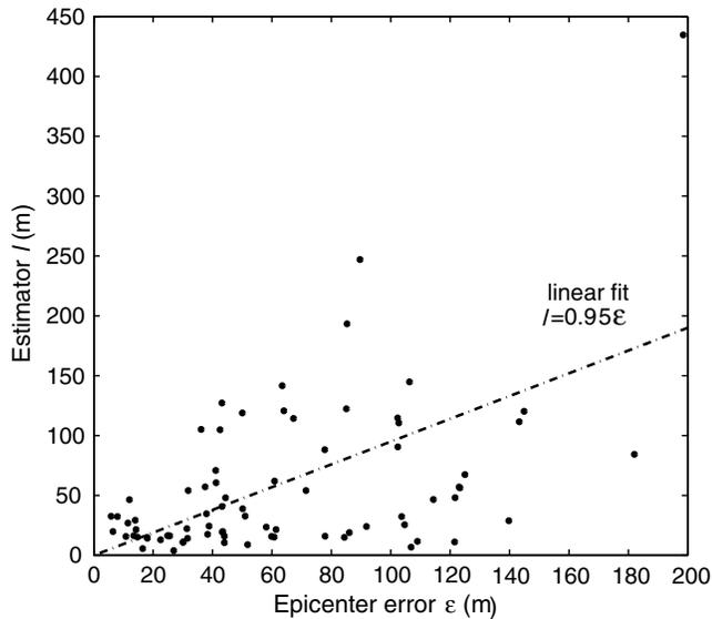
**Figure 7.** Epicenter location error  $\epsilon$  versus the distance  $l$  estimated from the area where  $C > 0.97C_{\max}$ . The dash-dot line represents the linear fit between these two quantities.
