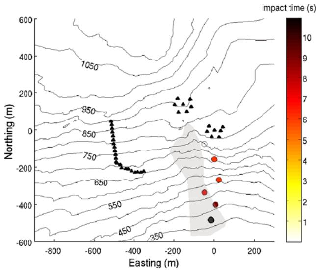
**Figure 10.** Location of impacts during the propagation of a rockfall that occurred on 6 June 2008. The color version of this figure is available only in the electronic edition.
