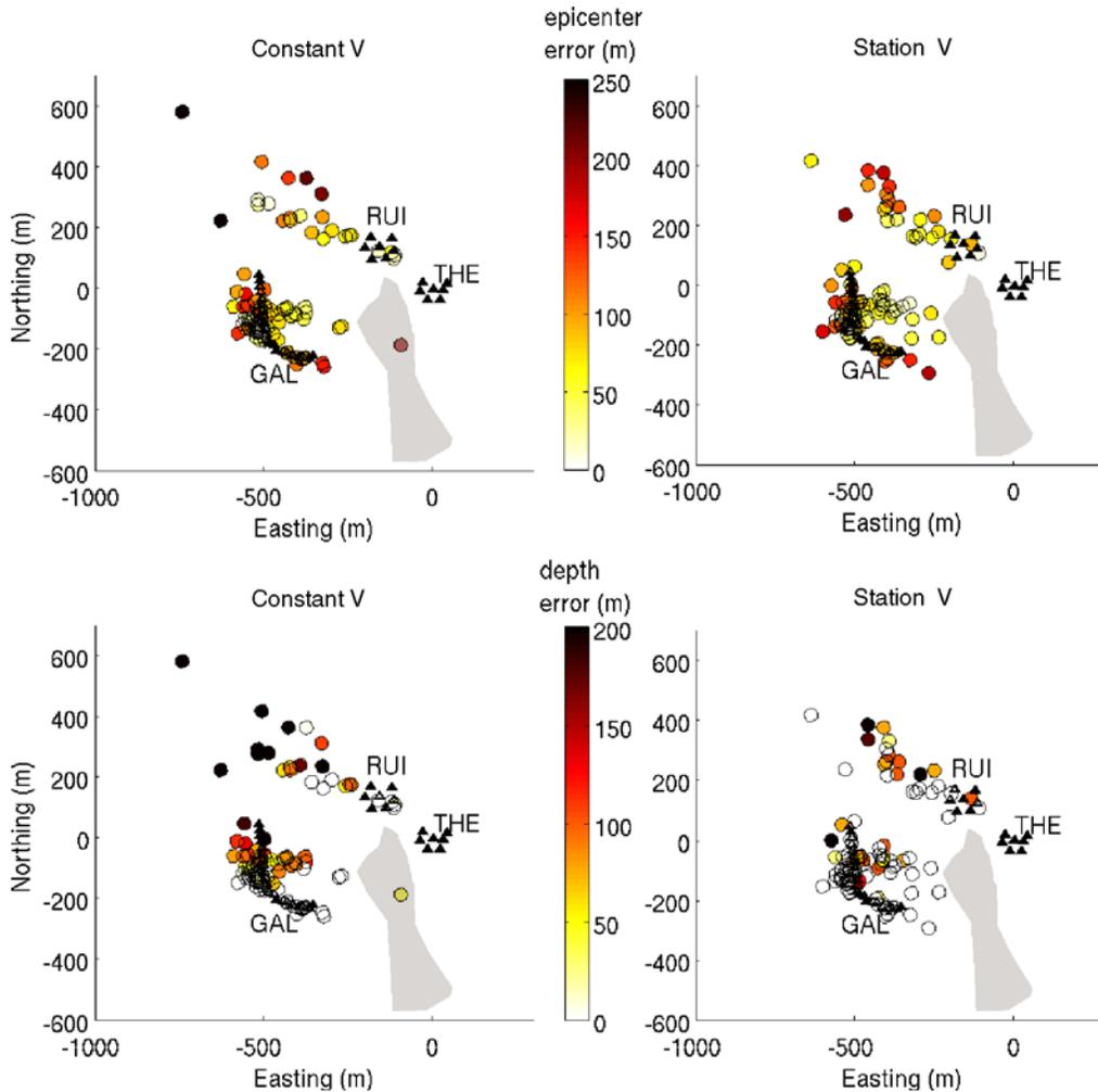
**Figure 6.** Location of shots (left) for a constant velocity and (right) for a station-specific velocity, estimated without fixing the depth at the surface. Top and bottom subplots represent epicenter and depth errors, respectively. The color version of this figure is available only in the electronic edition.
