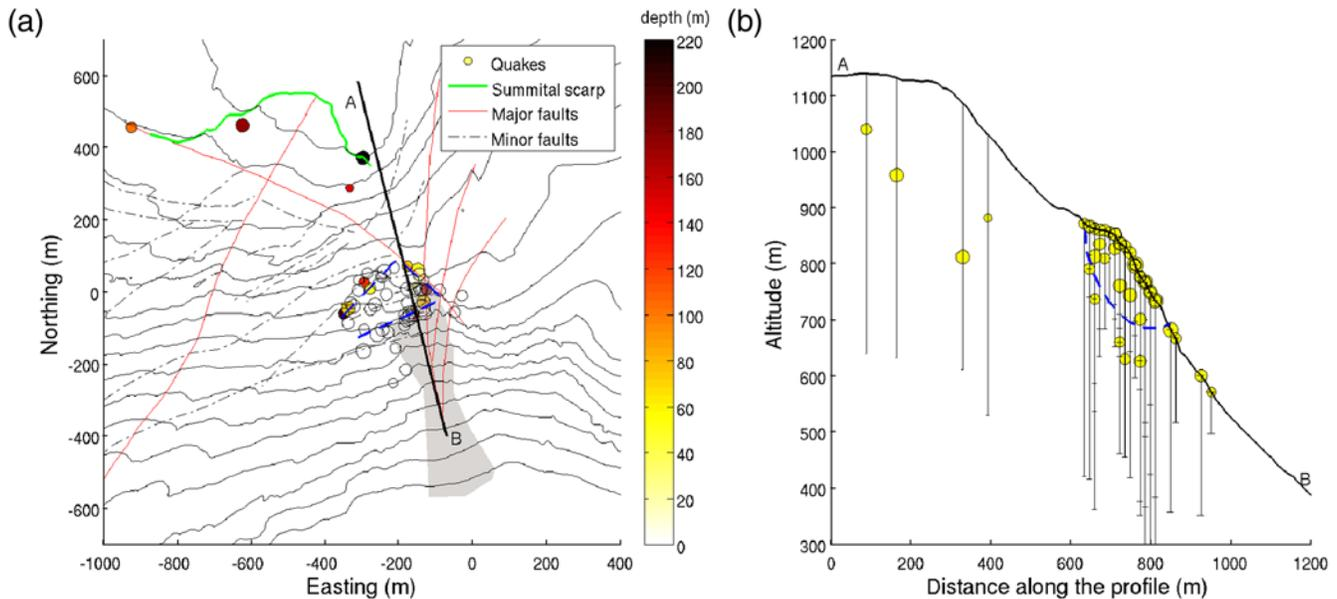
**Figure 11.** (a) Location of microearthquakes on a geological map. Microearthquakes are represented with circles sized by their magnitude. (b) Sources projected on the profile A–B. The dashed line represents the limit of the unstable area as estimated from the seismicity. The color version of this figure is available only in the electronic edition.
