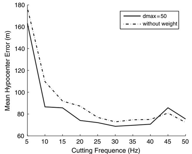
**Figure 4.** Mean location error for shots of June 2008 as a function of  $f_{\max}$  for two runs with or without weight ( $d_{\max}$ ).
