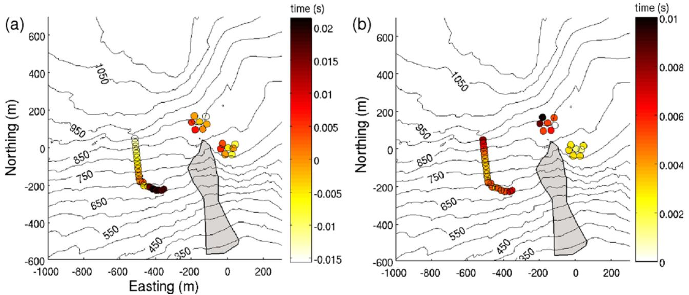
**Figure 3.** (a) Average value and (b) standard deviation of residuals between  $P$ -wave arrival times and theoretical time delays for shots. The color version of this figure is available only in the electronic edition.
