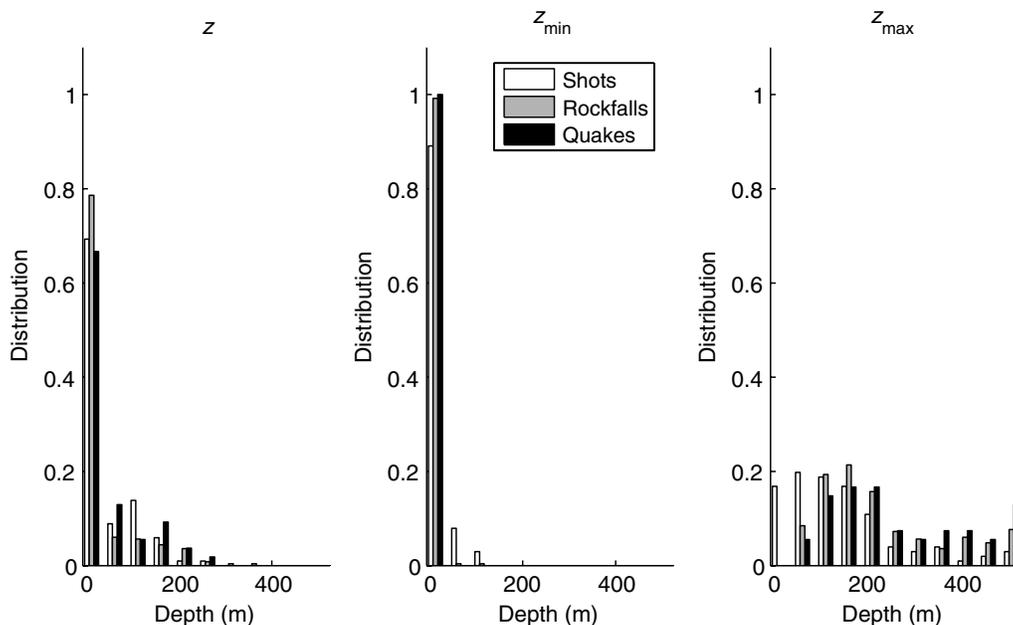
**Figure 8.** (Left) Distribution of depth, (middle)  $z_{\min}$ , and (right)  $z_{\max}$  for the different types of events. White, shots; gray, rockfalls; black, microearthquakes.
