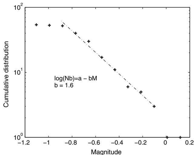
**Figure 12.** Cumulative magnitude distribution for microearthquakes.
