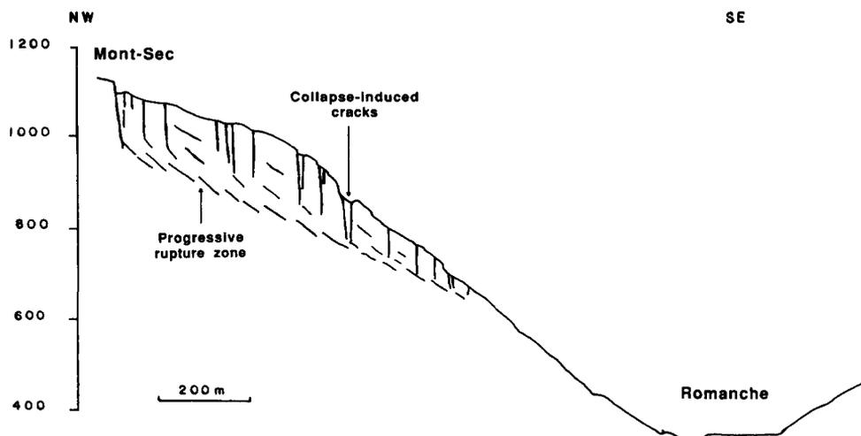
Fig.6. Sketch cross-section of the Ruines de Séchillienne site.
