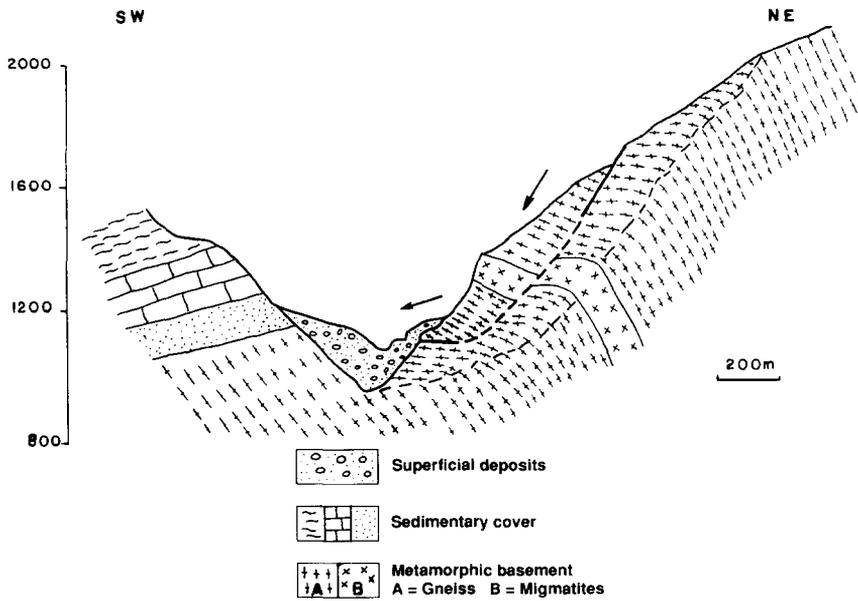
Fig.4. Geological cross-section of La Clapière landslide (after Follacci, 1987).
