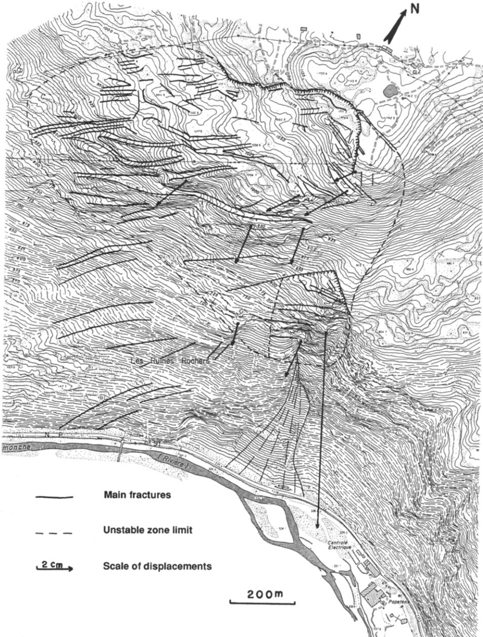
Fig.7. Direction of displacement vectors between February and November 1988 at the Ruines de Séchilienne site.
