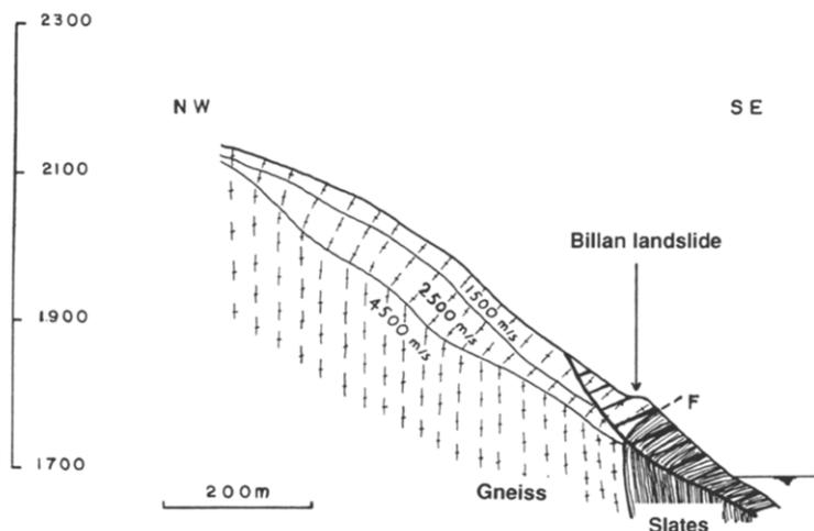
Fig.2. General slope profile of the Billan landslide (after Dubie and Guitton, 1988).
