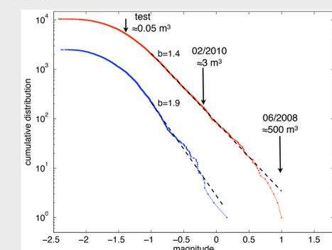
Fig 4: magnitude distribution for rockfalls and micro-earthquakes.
