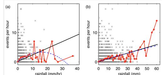
Fig 9: Rockfall rate as a function of (a) hourly precipitation and (b) antecedent rainfall  $P_c(t)$ . Grey crosses are the raw data while red dots show the data averaged over bins of precipitation. Black lines are linear fits of the raw data.
