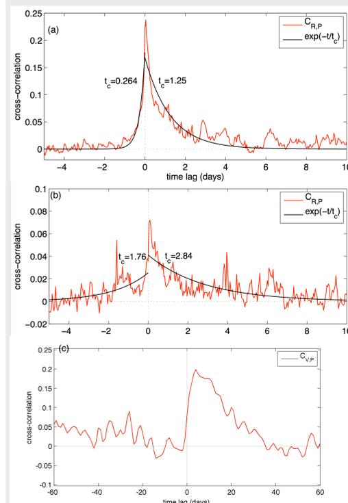
Fig 7: cross-correlation between precipitations and (a) rockfall rate (b) micro-earthquakes and (c) rockslide displacement rate.
