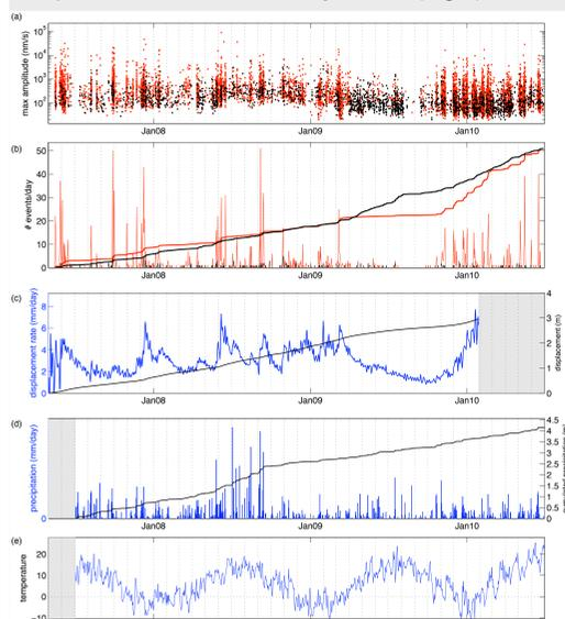
Fig 6: time series of (1) amplitude of rockfalls (red) and micro-earthquakes (black), (b) rate of events (c) displacement of target 635 (data from CETE Lyon) (d) precipitations and (e) temperature recorded at Luitel (data from LTHE).
