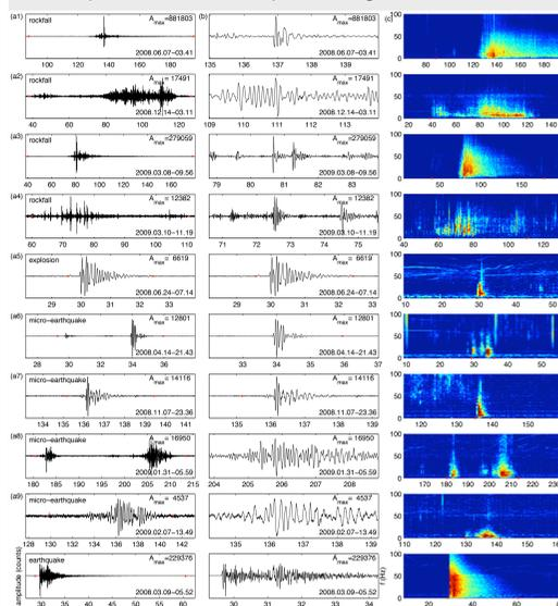
Fig 3: A selection of different types of signals. (left) Seismograms recorded by station THE and (middle) zoom for a window of 5 s around the peak of amplitude. (right) Spectrograms.
