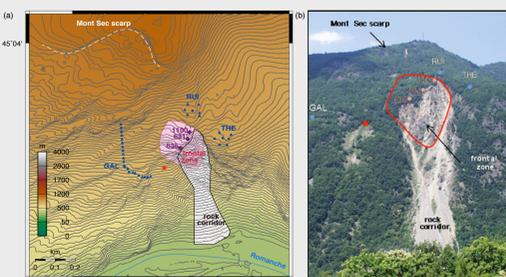
Fig 2: (a) Map of the rockslide and of the monitoring network: vertical sensors (circles) and 3-component seismometers (triangles) for the 3 stations. Also shown are the locations of 3 benchmarks of the displacement network (diamonds) and the location of a shot on 24 June 2008 (red star). (b) photo of the rockslide and limit of the most active zone (red contour).
