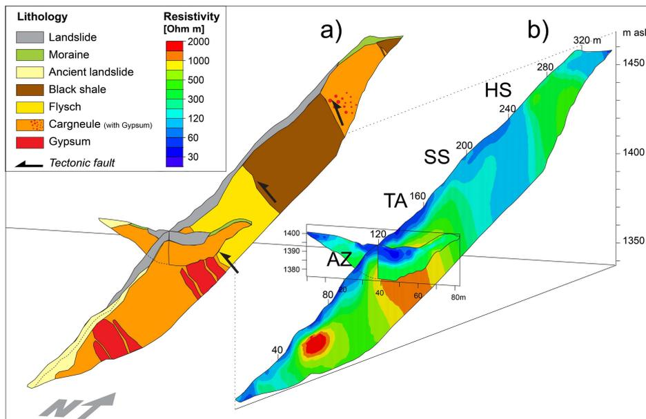
FIGURE 7.3 – (a) North-south geological cross section along the Pont Bourquin landslide, constructed from the local geological atlas (*Badoux et al. (1990)*) and the electrical images shown in Figure 2b. (b) North-south and east-west oriented electrical resistivity tomography profiles (see location in Figure 7.2). The head-scarp (HS), main secondary scarp (SS), transportation area (TA), and accumulation zone (AZ) are also indicated.
