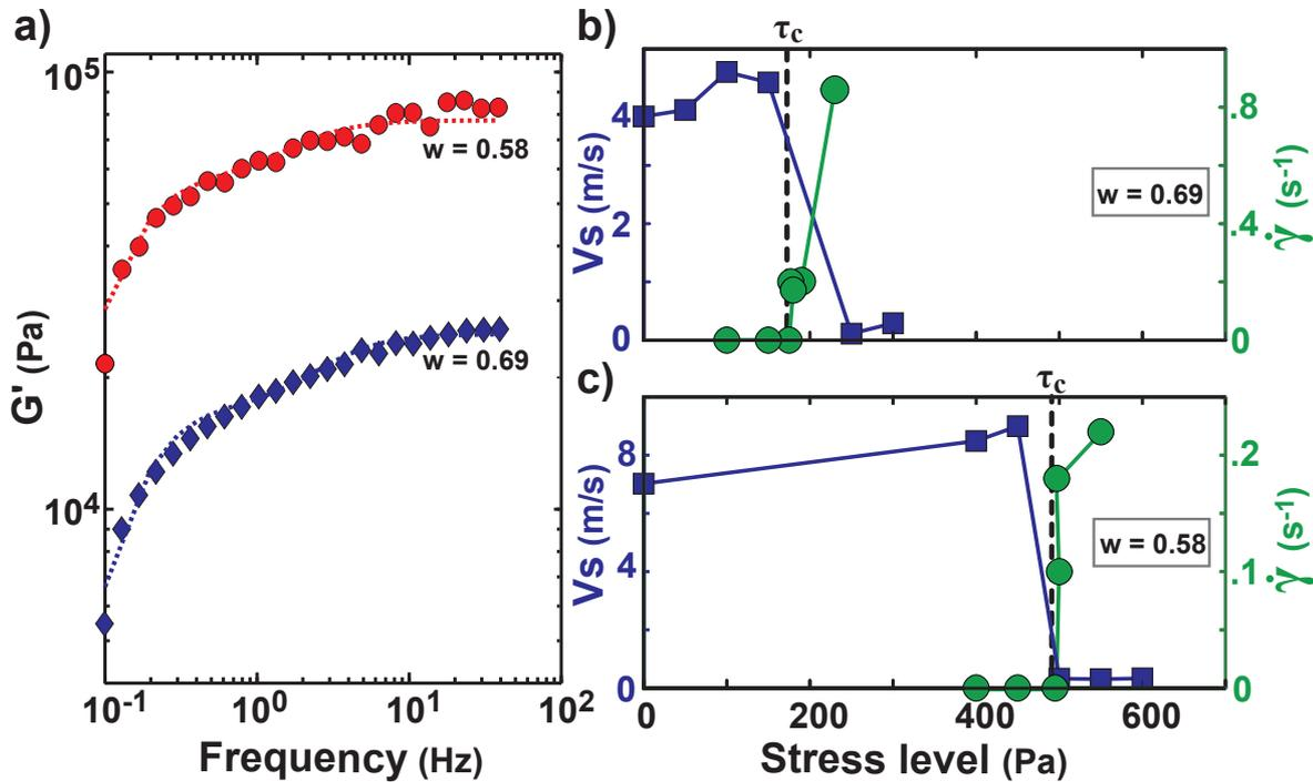
FIGURE 4.15 – a) Real part of the viscoelastic modulus ( $G'$ ) as a function of frequency for two samples at different water contents  $w=0,58$  (red circles) and  $w=0,69$  (blue lozenges) and at steady stress=0 Pa. b) and c) : Values of  $Vs$  (squares, oscillatory tests) and steady-state strain rate (circles, creep tests) as a function of imposed stress for the same water contents.
