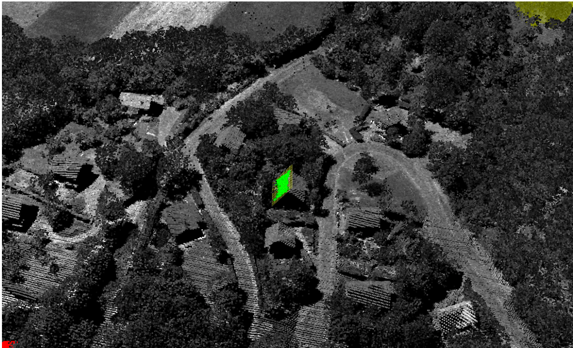
Figure 4.28: Perspective view of the 2006 Lidar point cloud showing the village of Mas d'Avignonet. The point brightness represents the reflectivity of the Lidar points. At one house a plane (yellow) is fitted into the roof using the green points.
