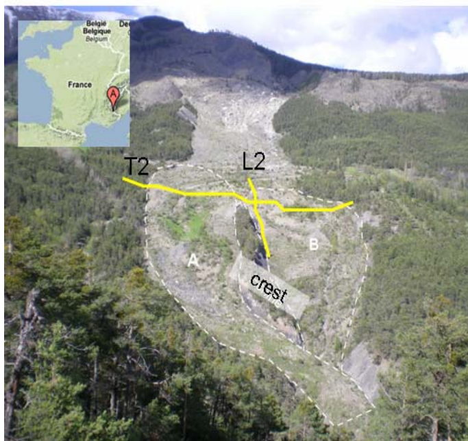
Figure 1. Location map and general view of the La Valette landslide. The two geophysical profiles (T2: transverse; L2: longitudinal) are shown in yellow; in the bottom part, the landslide shares into A and B.
