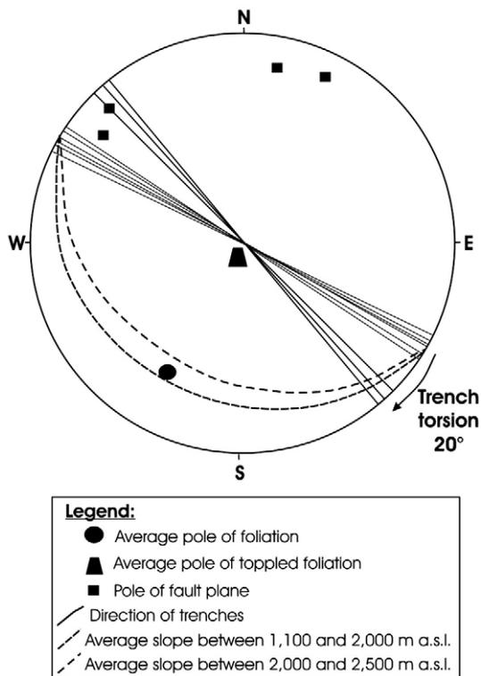
**Fig. 3.** Stereonet showing major structural features. (1): major faults; (2): foliation ( $60^{\circ}/040^{\circ}$ ); (3): toppled foliation ( $005^{\circ}/040^{\circ}$ ), (4): trenches ( $N110^{\circ}$  to  $N140^{\circ}$ ) and (5) slope direction. The black arrow indicates the trench flexure in the north-western part of the rock slide.
