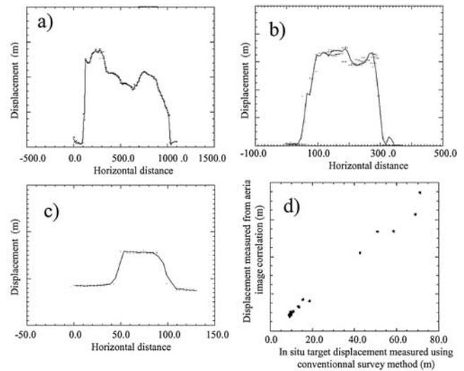
**Figure 3.** Displacement profiles (a) Crossing the landslide (b) Crossing the north-east lobes (c) Along the bottom landslide, (d) Correlation between in situ displacements measured by tachometry on targets located on Figure 2 and by correlation technique.
