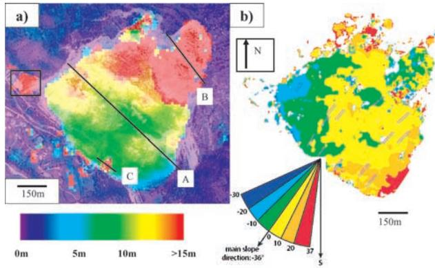
**Figure 2.** Displacement map obtained by correlation between aerial photographs acquired in 1995 and 1999. (a) Horizontal amplitude (b) Orientation. Displacement vectors measured on ground by laser telemetry (pink arrows) and by correlation (blue arrows).
